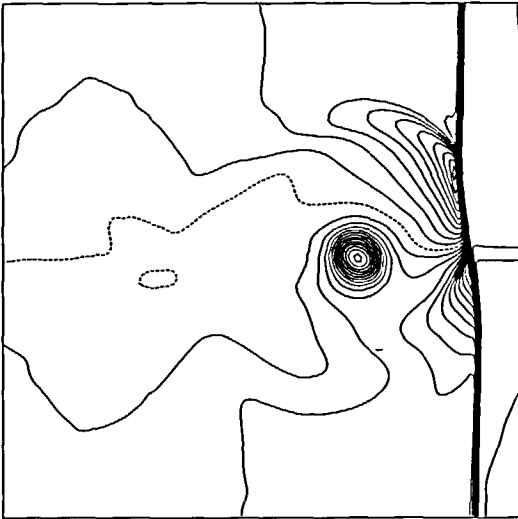
Figure 11 Shock vortex solution ( t=1.00 ) using 500 \times 120 cell stationary grid
