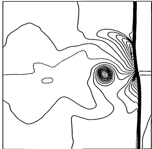
Figure 10 Shock vortex solution ( t = 1.00 ) using 300 \times 120 cell stationary grid
